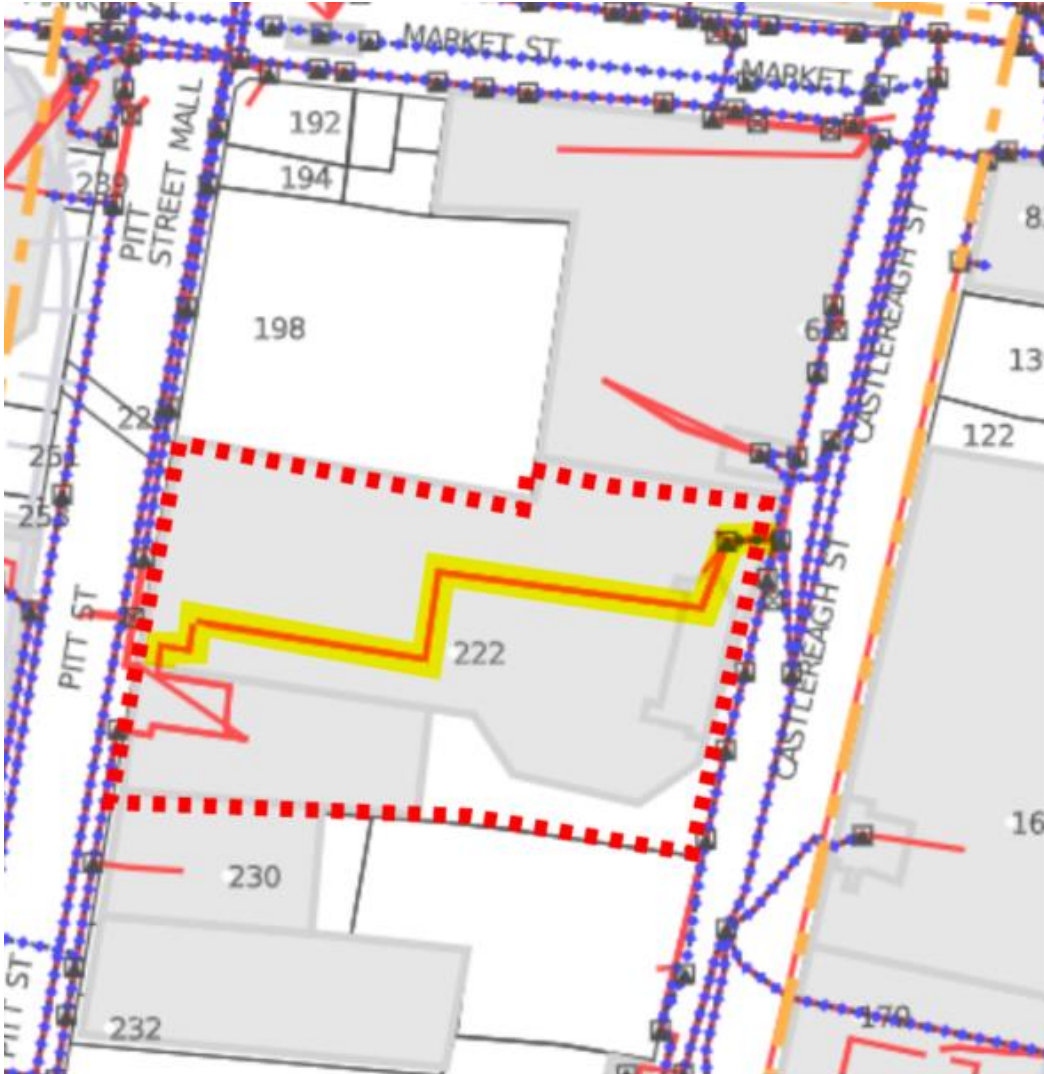
Figure 5: Optus existing Communications Services adjacent the site
