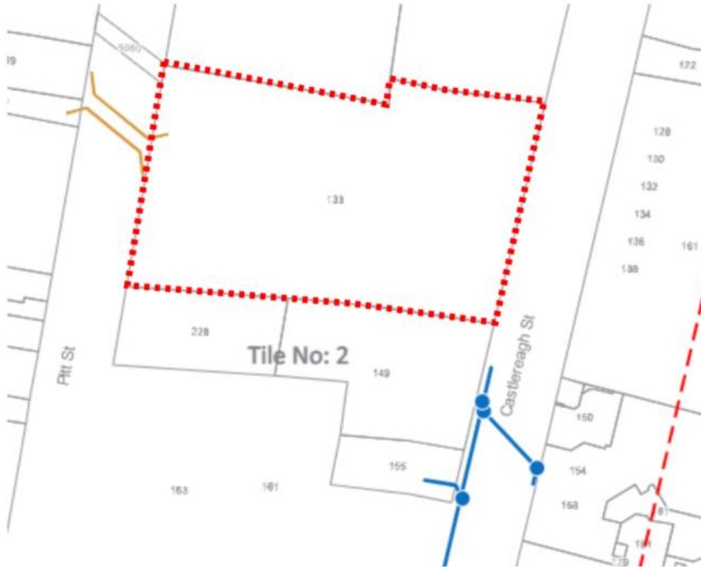
Figure 8: Vocus existing Communications Services adjacent the site
